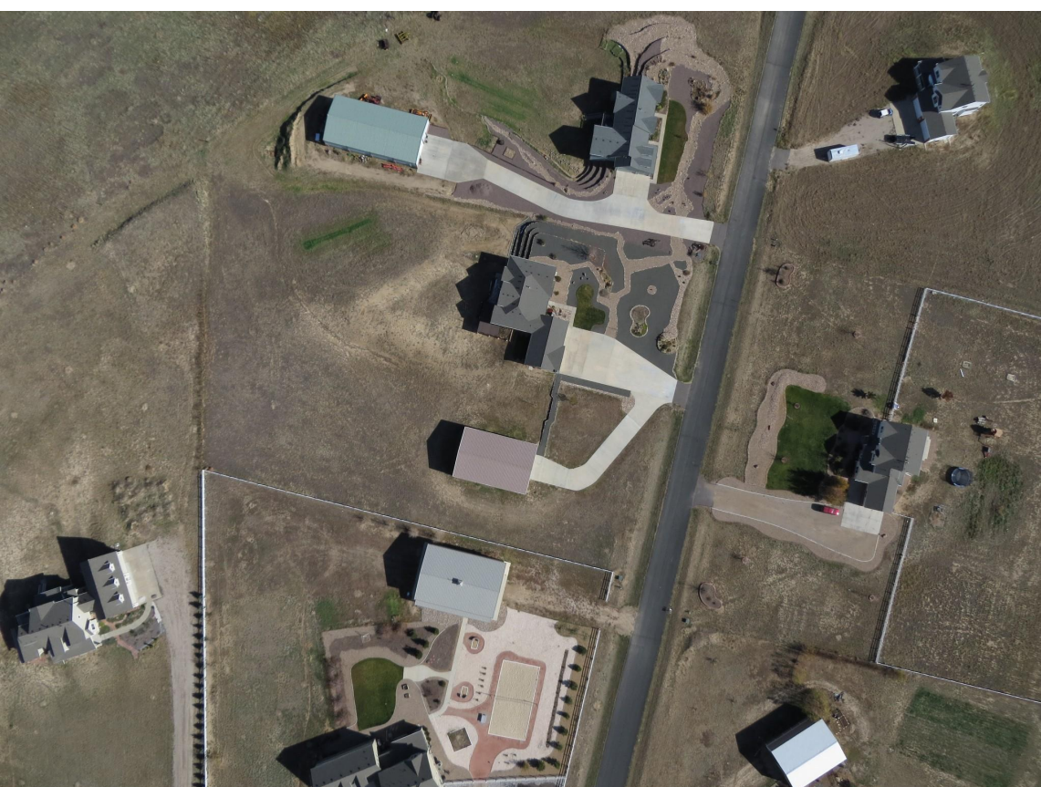
Falcon UAV Example Imagery from Canon SX260HS at 200 meters. 6.7 Ground Sample Distance (GSD)
